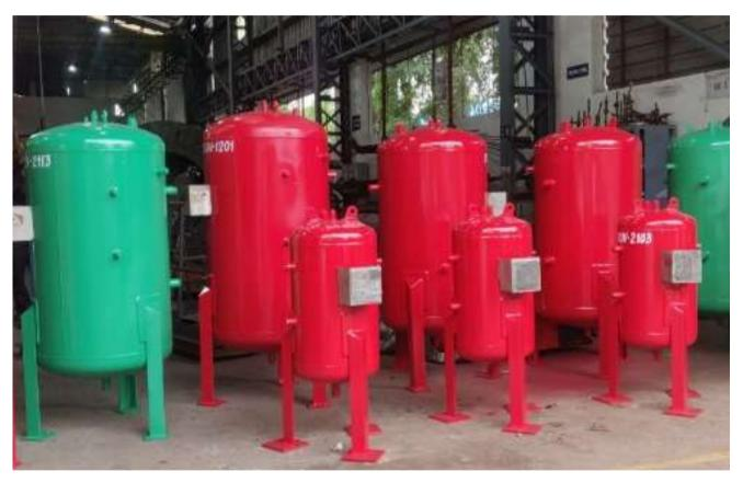
12 Air Receiver of capacity 1m<sup>3</sup> & 0.27m<sup>3</sup>
